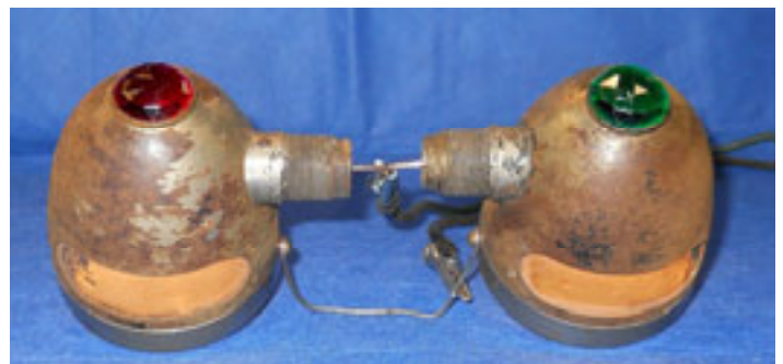
The side lamps that John Lewis sent Joe Leaf. [Ed: Note that Joe powered the lamps to make it easier to see the courtesy light and colored jewels.] (Joe Leaf)
