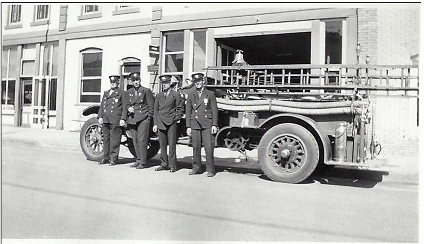
A photo from 1942 when the KisselKar was taken out of service. The hoses are draft (intake) hoses for the Waterous 300 GPM pump that was installed in 1926. This photo was taken in front of the firehouse out of which we still operate.
