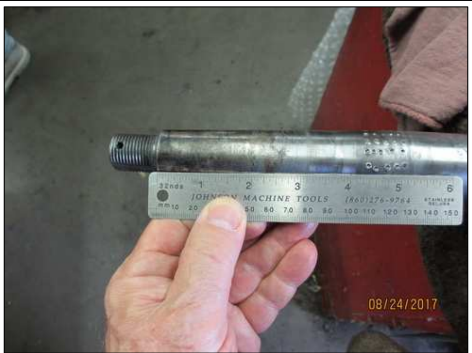
Doug is holding a steel ruler along the tapered outboard end of the right axle. Notice the punch marks used to expand this axle to mate the inner race of a wrong bearing.
