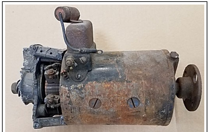
The deteriorated, original equipment Remy 912B
